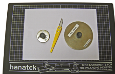
Sample template cutter for 50mm and 115mm \varnothing included with instrument. Suitable for low volume testing.
