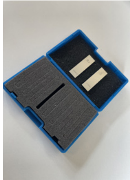
Traceable 2000 µm and 500 µm checking gauges
